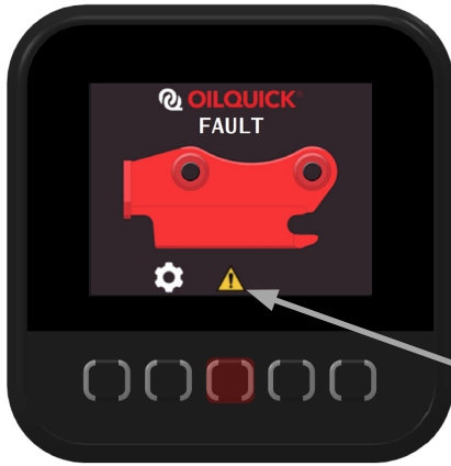
Coupler Open, Fault Active
