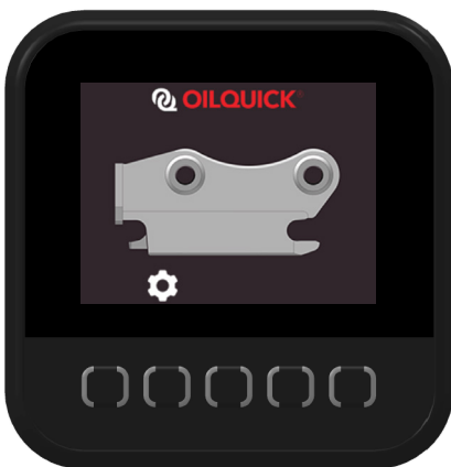
Locked, Insufficient Pressure
