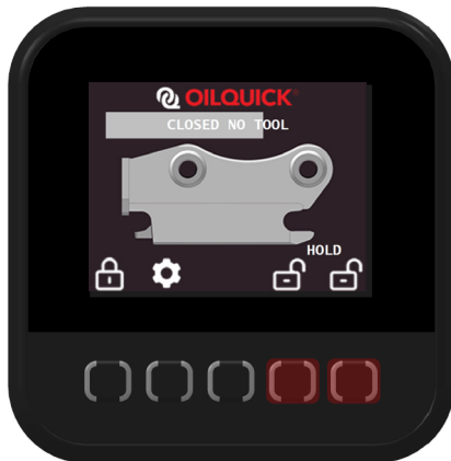
Opening From Coupler Closed Without Tool
