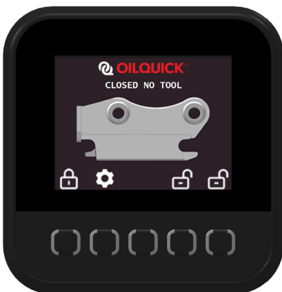
Coupler Closed Without Tool
