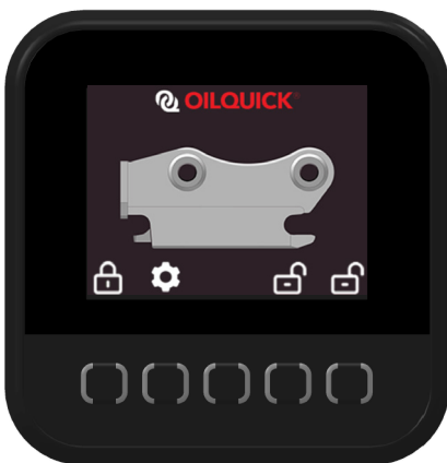
Locked, Insufficient Pressure
