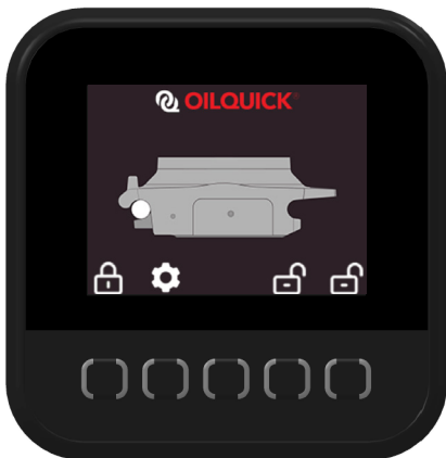
Locked, Insufficient Pressure
